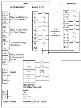
Terminal Connection: For Output Relay, Fault Input, Remote Keys,
